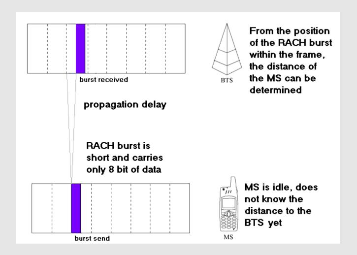
MS sends a RACH burst to access the GSM network (Channel Request)
