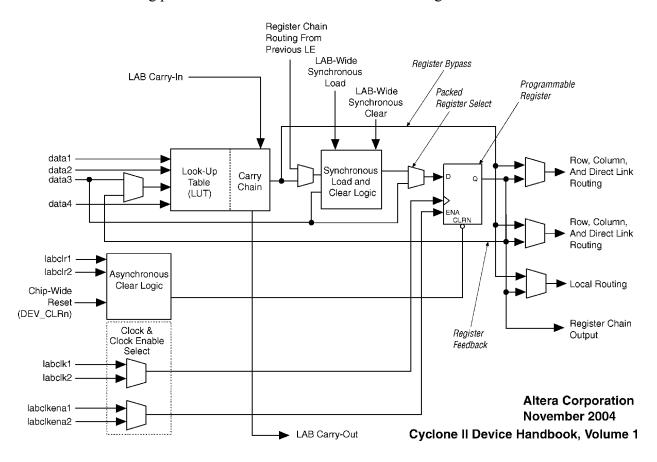
As can be seen a Logic Element looks rather complex. But its main operation is quite simple: To store states it has a programmable Register. A clock allows the register to switch state depending on the clock and the input signals. The Lookup Table provides combinatoric logic.
