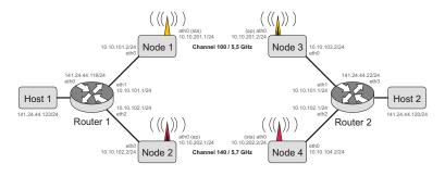
Optimization of a point-to-point link Second WLAN link for full-duplex traffic flows
