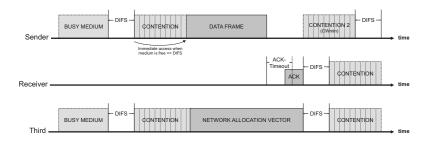
• Contention phase: Wait a random number of time slots  $[0;2^{CW} - 1]$ . Start with  $CW = CW_{min}$ . Double CW by every retransmisson attempt, till  $CW_{max}$  is reached.
