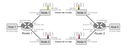
Optimization of a point-to-point link Second WLAN link for full-duplex traffic flows
