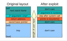
Figure 1. Stack before and after a stack-based arc injection.
