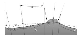
Figure 2: Figure of the Geoid. 1 ocean, 2 ellipsoid, 3 local plumb-line, 4 continent, 5 geoid. Source: en.wikipedia.org/wiki/File:Geoida.svg
