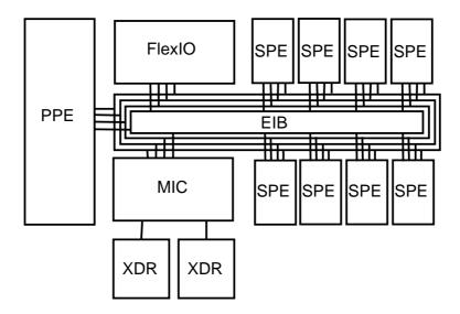
Figure 1: Cell Architecture
